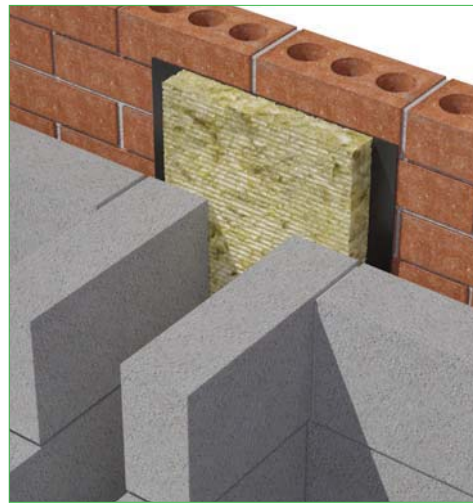
Junction between external cavity wall & party wall
