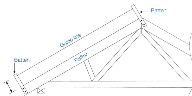
75mm + thickness of roof covering
